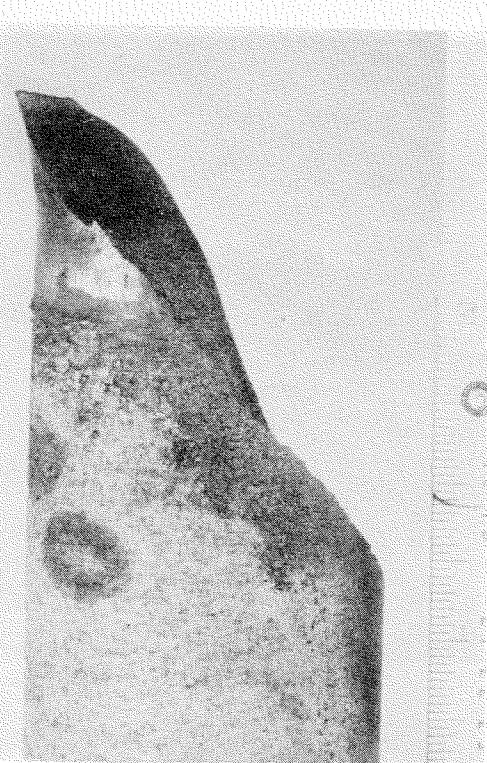
Fig. 3-16 Photographs of Fractured Specimen of Sea Water Corrosion Fatigue Test
