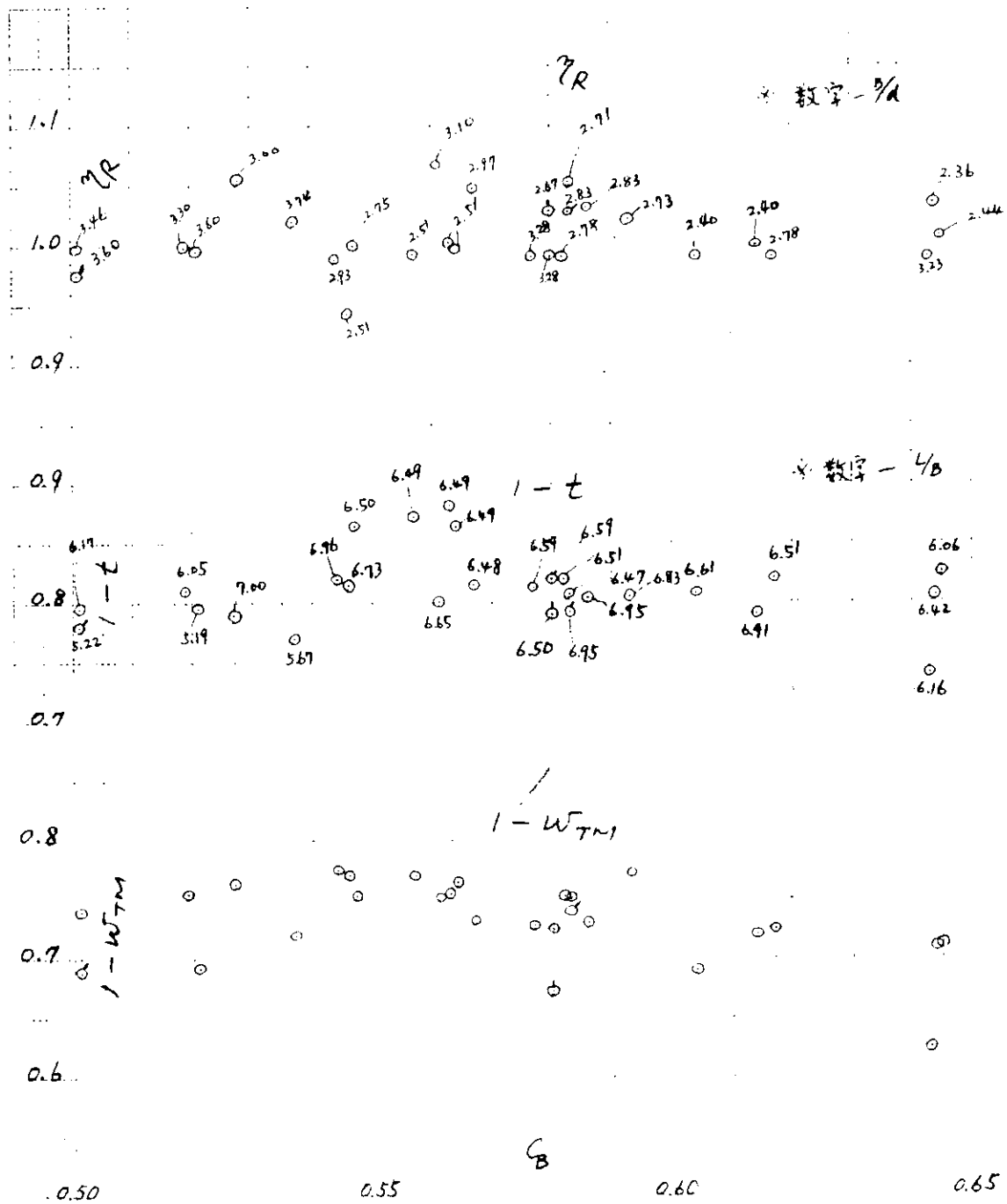
Fig. 2.4.12 C_B \sim SELF PROPULSION FACTORS ( F_n=0.28 )
