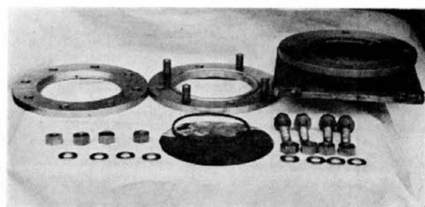
Fig. 2.14 Parts of Maximum Water Pressure Gage
